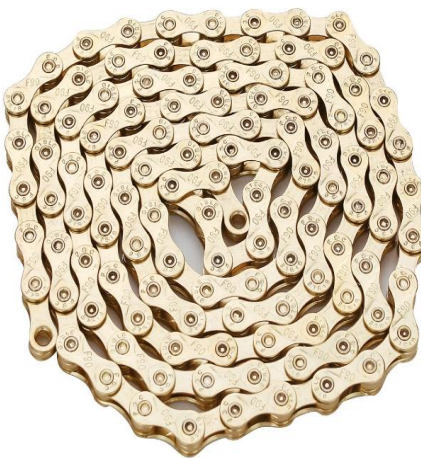
FSC F90 9 speed chain Gold,1/2"X 11/128",116L
